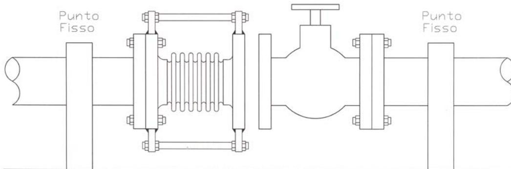
DISMANTLING JOINT WITH DISMANTLING TIE RODS AND PRESSURE BEARING TIE RODS
