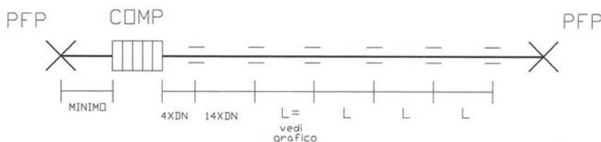
The distance of the first axial bind has to be 4 times the nominal diameter of the pipeline, the second one 14 times and from the third one in then it is necessary to refer to the chart restored to page 7 summary from the rules E.J.M.A..
