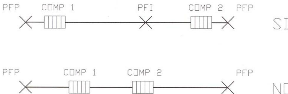
Besides it is a good rule to install the expansion joint as close as possible to the anchor point, giving back in this manner one of two ends practically fixed, increasing the total stability of the pipeline. Another fundamental detail for the correct installation of the expansion joints, is the predisposition of the axial binds, that give guarantee of perfectly axial motion of the pipeline, avoiding unwanted damages.
