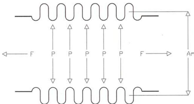
You consider that the presence of the back push, is cause of installation's problems, when in decisive areas of an installation, is not possible to realize anchor points supplementary to contain it. For this reason is possible to build expansion joints, that thanks to their special construction, can to contain autonomously this force, without to need of other anchor points.
