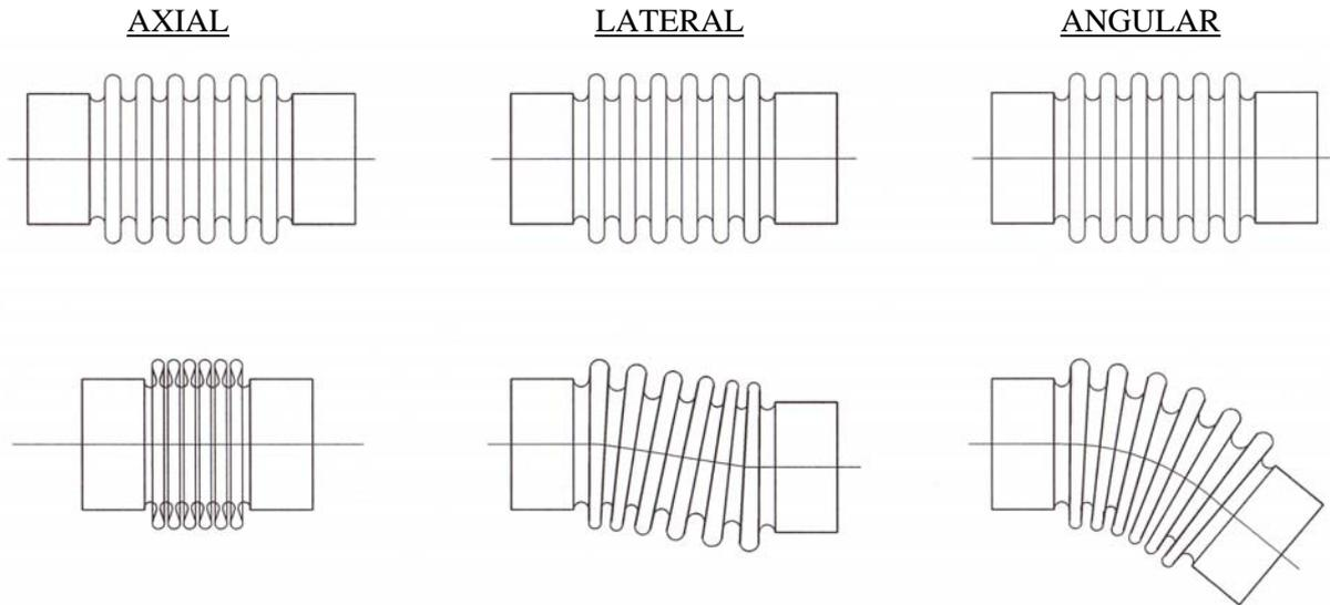
Normally these expansion joints are used with pipeline where because of the variations of temperature, expand, provoking (if done not compensate for note) of the disruptions either of the deformations to the same pipelines or to the rigid parts to are connected.
