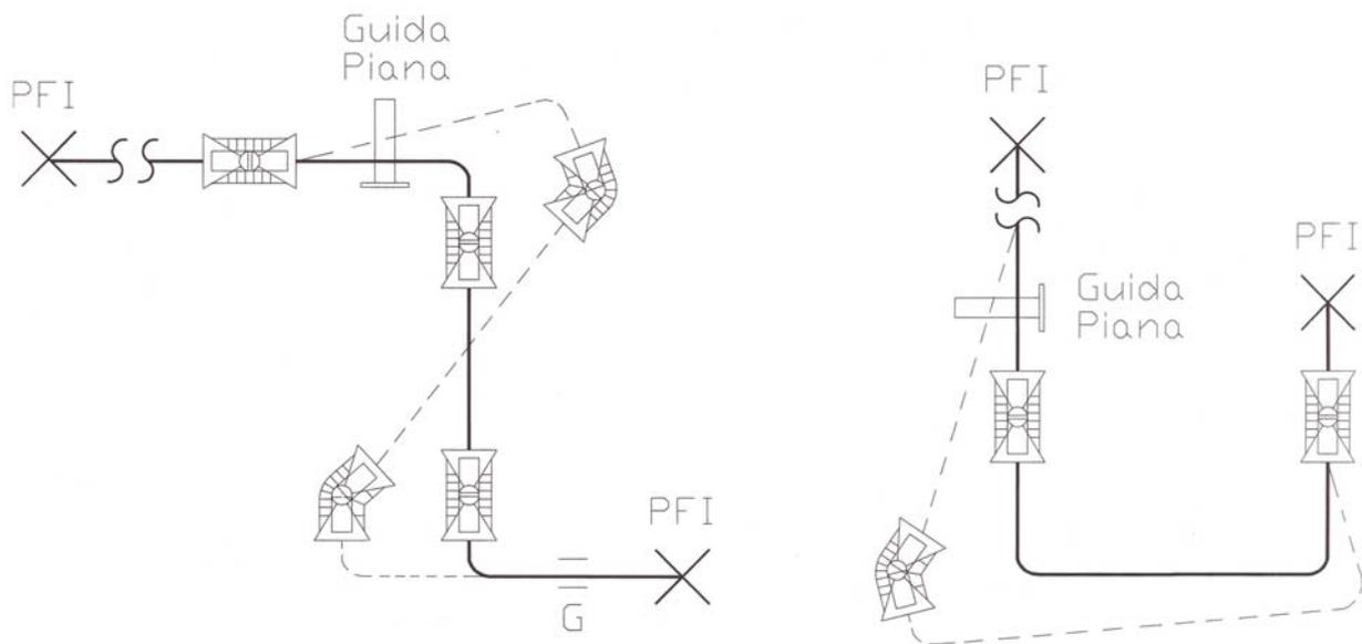
When they use themselves the angular expansion joints in these configurations, is necessary to arrange (in proximity of the same expansion joints) of the plain binds, to agree bendings to the rigid pipeline, because of the final composition of the movements carried out; the better solution consists to use the configuration that expects 3 expansion joints.
